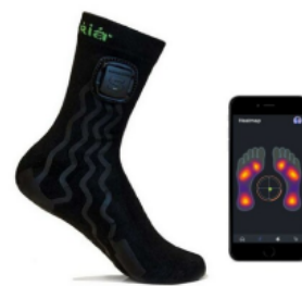
Sensoria textile sensor infused sock and balance data heat map
